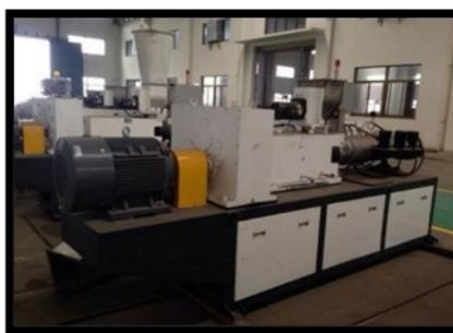
Fig 2: Twin screw extruder
