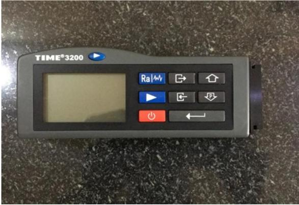
Fig 3: Surface Roughness Tester 3200
