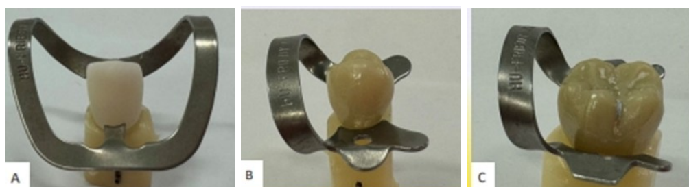
Figure 1. Rubber Dam Clamps on Crowns. A: Anterior 5Y zirconia crown cemented to die with RDC in place B: Premolar 4Y zirconia crown cemented to die with RDC in place. C: Molar 3Y zirconia crown cemented to die with RDC in place.
