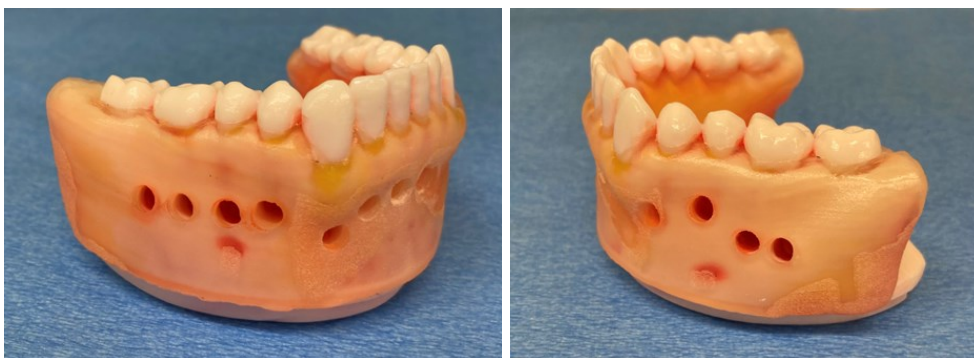
Figure 4. Root end resection sites on TrueJaw Endosurge models.
