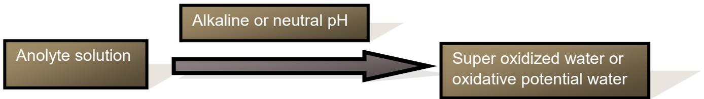
Principle: It is based on the principle of “Flow-through Electrolytic Module” or FEM which means transferring liquid into a metastable state via anode and cathode through the use of an element.<sup>10</sup> It is producing solutions (Superoxide water or oxidative potential water) that have high sporicidal or bactericidal activity.
